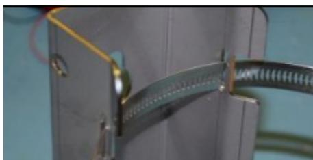
Slide the Tamtorque through the two gaps in the bracket and then around the post to which the sign is being fixed onto.
