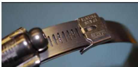
Before fully tightening the fixing in position, use the small clip to hold the excess band neatly in position.
