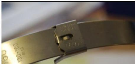
Begin by making sure that a small clip is found on the Tamtorque fixing.
