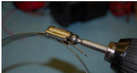
While pushing the fixing in this position, pick up the drill with the Tamtorque bit and screw clockwise into the hole as shown on the left. This should then start to tighten around the post.
